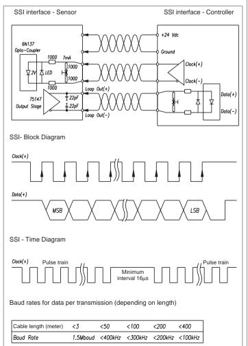
Max. frequency: 2Mhz Min. frequency: 50Khz
